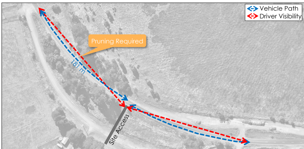
Figure 34 Safe Intersection Sight Distance Assessment
